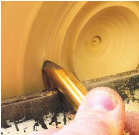
▲ Pic.10 Once he's finished the back of the bowl he remounts it using the spigot and starts the hollowing. Unlike a normal bowl a stem will be left in the centre
